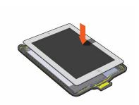
2 SLIDE THE CASE FRONT ON AT AN ANGLE, HOOKING THE BASE ON FIRST
