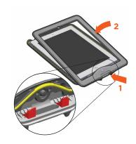
FIRMLY SNAP FRONT AND BACK OF CASE TOGETHER
