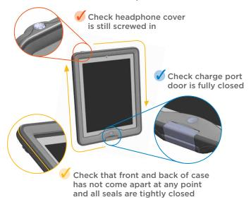
AFTER MAJOR IMPACTS: IT IS HIGHLY RECOMMENDED THE FIRST TIME INSTALLATION PROCEDURE IS PERFORMED TO CHECK THE INTEGRITY OF THE CASE BEFORE EXPOSING TO WATER
