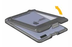
This ensures the slide hooks are cleared when iPad is removed
