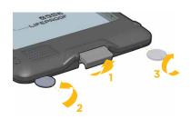
Do not bend the case back and remove in a single motion
