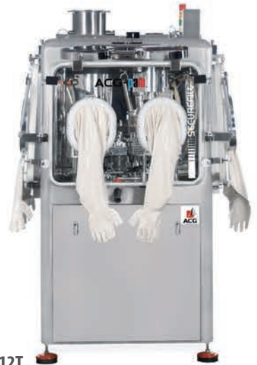
AF 90T (Tamping) Upto 90,000 capsules/hour (150,000 capsules/hour variant also available)
