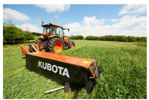
Kubota introduces the DM1000 and DM2000-Series side-mounted disc mowers with a working width ranging from 5'6" up to 10'6". A fully-welded cutterbar with overlapping C-channels sets Kubota disc mowers apart.
