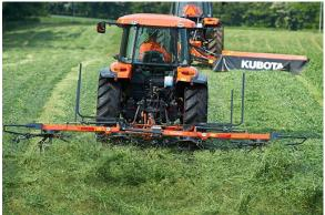
Kubota introduces the TE4052T rotary tedder, designed to optimize performance for producing dry hay. The pull-type design with a low weight of 904 lbs. is ideal for low-horsepower tractors or on hilly terrain.
