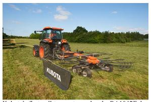
Kubota's first pull-type rotary rake, the RA1042T, has a working width of 13'9" and is fitted with 11 tangential tine arms and four double tines per arm and is ideal for low-horsepower tractors.
