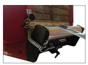
**Backside Web Reader.** This attachment repositions the mark sensor to read print marks on the backside of the web, and is necessary for front-to-back registration on a second pass.
