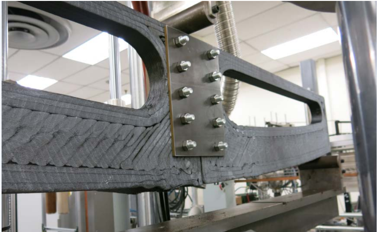
Figure 9: Successful Three Point Bending Test of Roof Assembly
