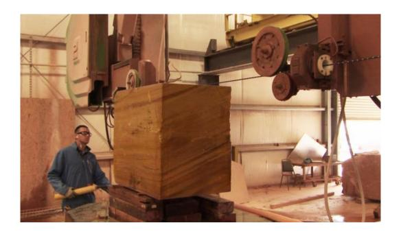
Advanced masonry technology was utilized to cut the meta-quartzite planters.
