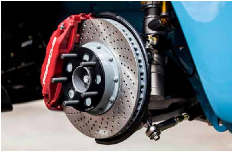
Singer Brembo™ Big Brake Upgrade
