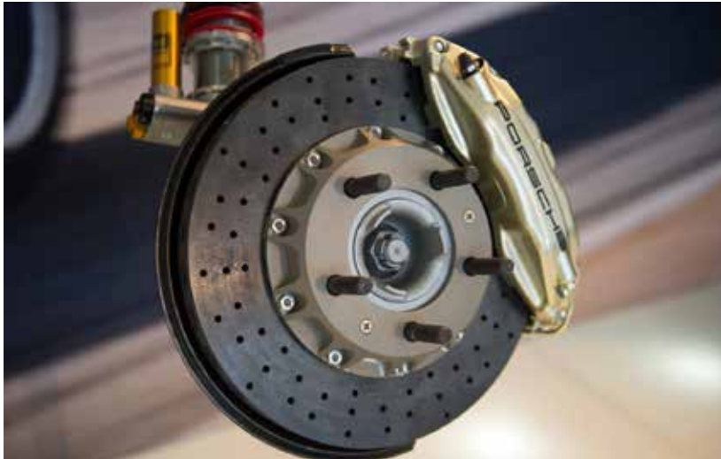
Carbon Ceramic Rotors with Big Brembo™ Calipers in Special Color
