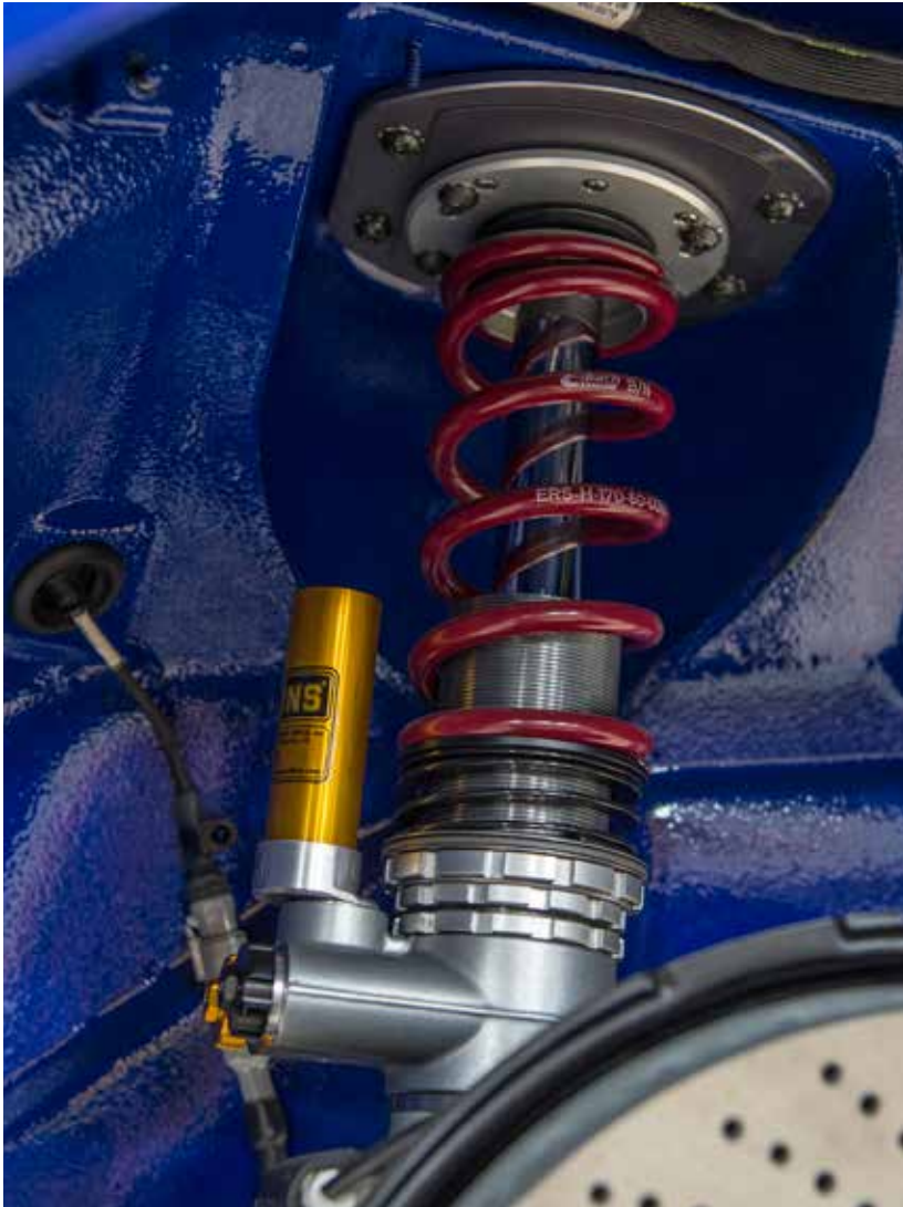
Ohlins™ Sport Adjustable Suspension
