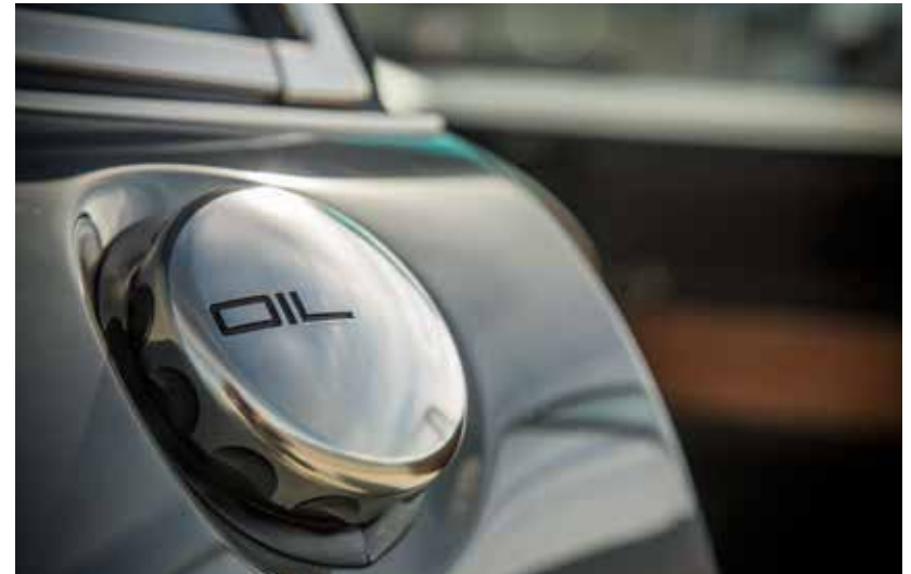
External Oil Cap Located in Rear Fender
