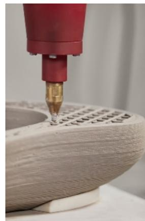
Like much of Arsham's work, Rock.01 is an homage to time. Comprised of 3D-printed vitreous china and hand-poured brass, the sink's vessel blends modern-day technology with Kohler's nearly 148-year manufacturing legacy into what can only be described as functional high art. The effects of time are reflected in the patina of the brass "rock" and achieved through a forced coercion process.
